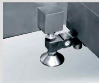
systemy wagowe w masownicach weighing system in tumblers
