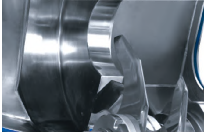
Narrow knife cover for improving the quality of meat stuffing
